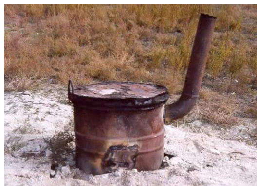
Fig. 4. Photograph of simple incinerator used for the combustion of healthcare wastes in a developing country.
